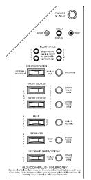
**LIGHTS AND SWITCHES** are provided to display boiler operating status, to indicate certain room and boiler fault conditions and to allow manual control of boiler functions for routine maintenance and troubleshooting.
