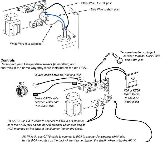
has its PCA mounted on the back of the steamer (<u>not</u>on the shelf). When using the AK I jack to create a system, DO NOT connect any controls or sensors to this same steamer!
