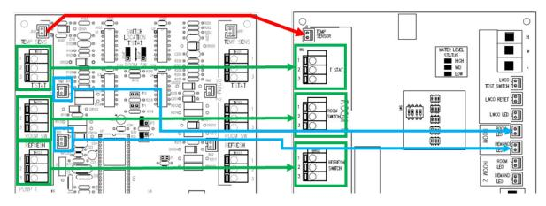
Move **Room 2** control wires and room temperature sensor cable if installed. Move room status LED cables as shown:
