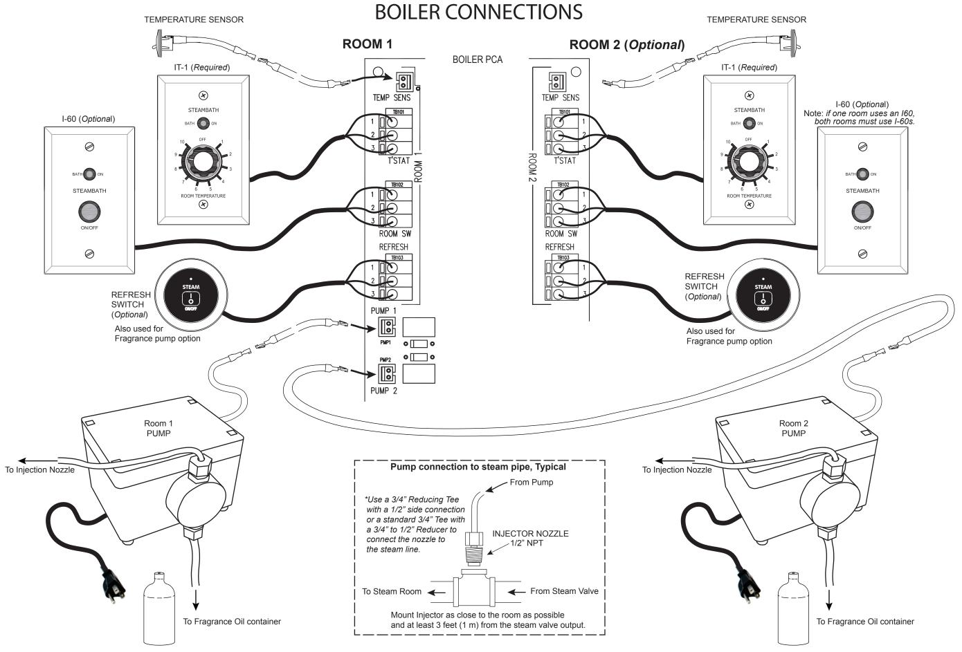
Note: the pump cycle will start whenever the Refresh switch is pressed (while the switch's light is lit)
