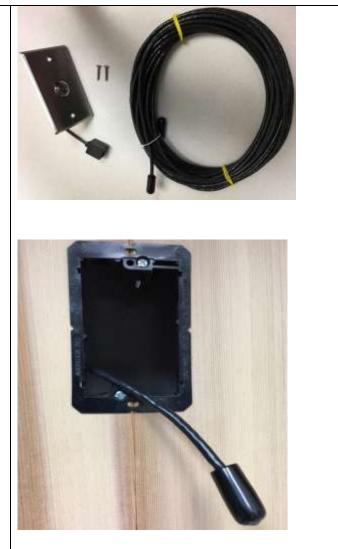
3. With the boot removed, insert the male RJ-10 connector into the female receptacle of the External Switch, as shown.
