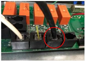
• There may be a piece of tape covering the Ext. Switch receptacle. Remove this tape prior to installation of the CAT5/RJ-10 cable.
