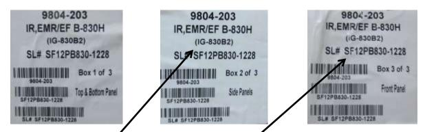
Box label will indicate the *model* of the room and the room *serial number*, the label will also give you the box number and the internal contents. (*Note: the above labels are samples only.*)
