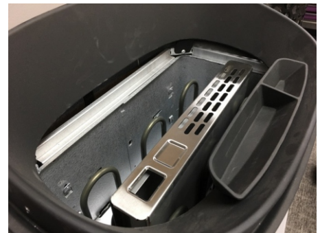
BWT tank, tank lid, and the vent cover installed.
