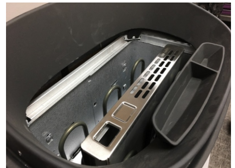
BWT tank, tank lid, and the vent cover installed.
