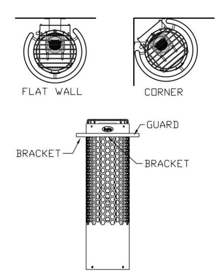
Note: Recommended height for heater guard brackets is 1-2 holes from top of heater.
