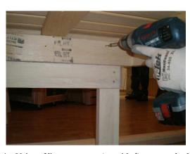
Step 4: Using 2" torx screws (provided), secure the bench to the arm rest assembly. Do this from underneath as shown above.
