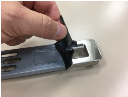
Remove plastic film from the BWT cover before placing in heater.
