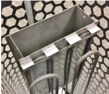
BWT tank hangs on the top of the heating elements.
