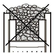
Placing the stones, a cross-section of the heater stone compartment Place the stones loosely, so there will be enough space between the stones.
