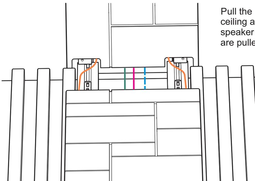
Pull the cables to the led lists up on the ceiling as shown. The cables to the speaker and possibly to the control panel are pulled up in the middle.
